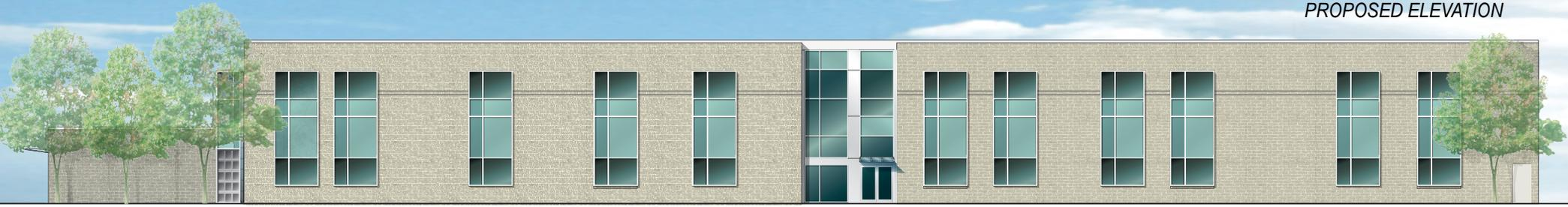
The brick veneer was removed between the existing 1st and 2nd floor windows to create a new single glazing element.
