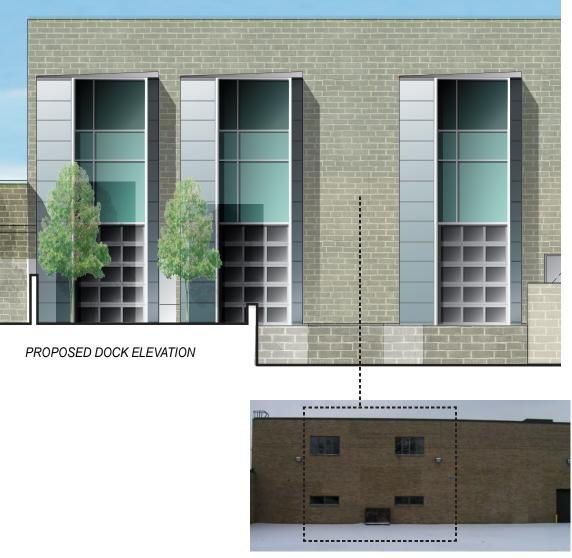
Angled additions to the building cleverly provide the potential for truck docks if needed by a future tenant. The replacement of the lower level of glazing with overhead doors and the excavation of dock ramps convert executive office space into loading docks without compromising the professional appearance of the building.
